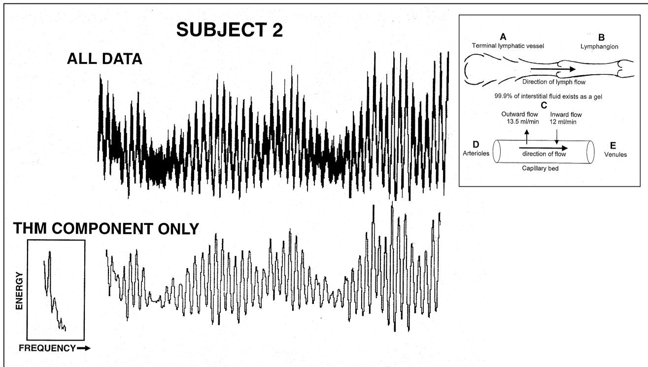
**Figure 4.** Inverse Fourier transform time-domain spectra from subject 2; top spectrum, all frequency domain data used in the inverse computation; bottom spectrum, only the frequency component lying below 0.5 cycles/sec (30 cycles/min) used. The bottom spectrum is the THM oscillation. The insert box shows that portion of the Fourier transform spectrum used to compute the inverse THM spectrum (see Figure 3).
