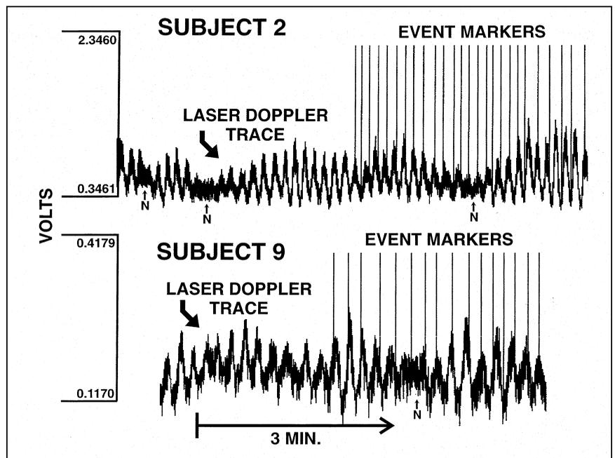
**Figure 1.** Compressed laser-Doppler flowmeter relative blood velocity (waveform) and flexion-extension records (vertical event marks) from two subjects (N, interference nodes).
